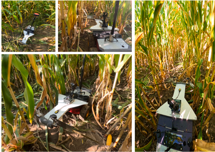
Fig. 17. Blind Navigation in a Cornfield. The blind navigation system is a novel system sensing modality that can be deployed to assist in navigating through a messy rugged environment, particularly where vision alone is insufficient.
